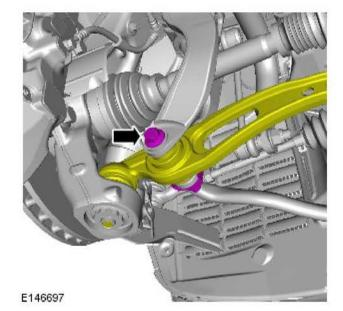
5. Lower the front left suspension lower arm to access the rubber bush.
