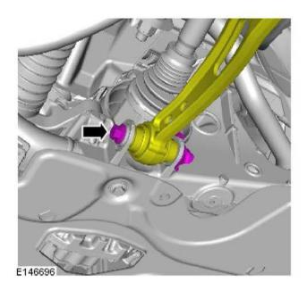
4. CAUTION: Nuts and bolts must be tightened with vehicle at normal ride height.
