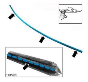
5. Install the upper windshield finisher, ensuring it is located correctly.
