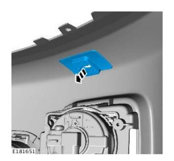
**5.** Remove the adhesive pad from the right-hand headlamp washer jet mounting plate.
