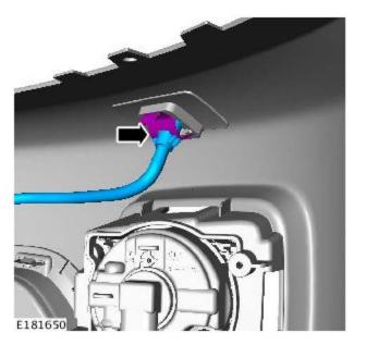
Remove the right-hand headlamp washer jet mounting plate.
