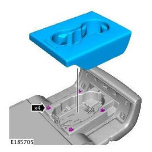
**3**Remove the second row seating center armrest operating handle retaining screws.
