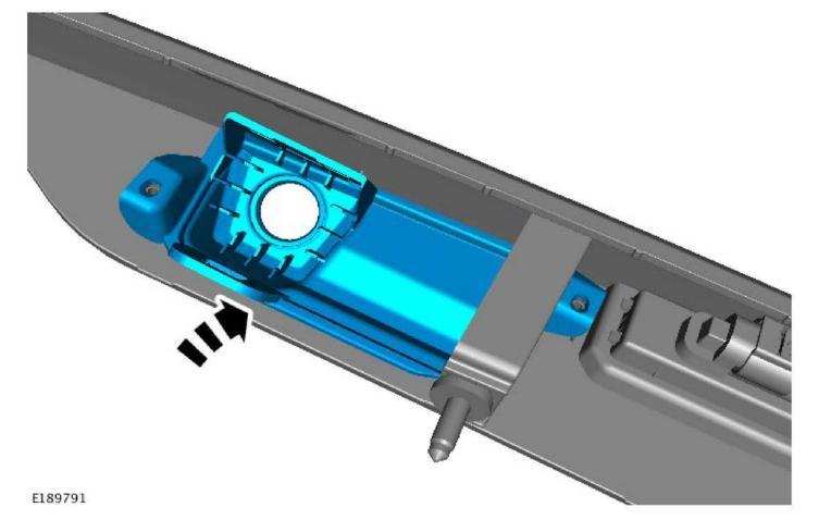
5. Install the two rear camera bezel screws.
