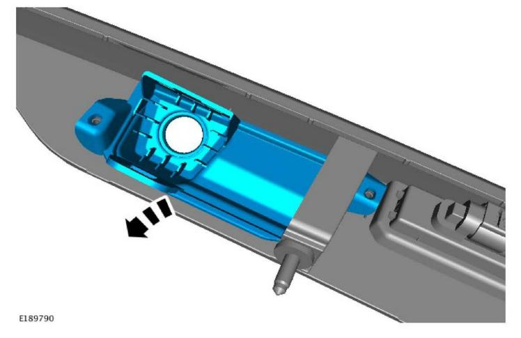
4. Install the new rear camera bezel.
