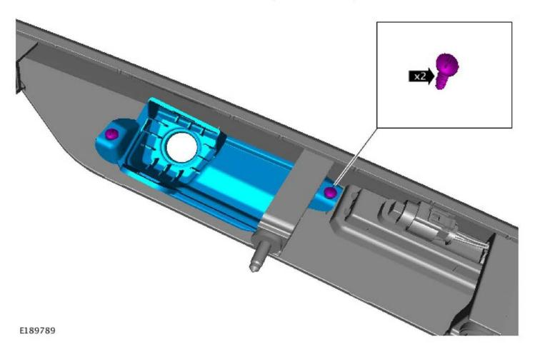
**3.** Remove the rear camera bezel.
