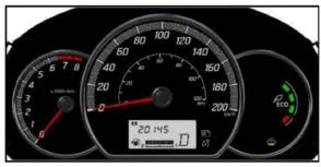
New combination meter display with constant illumination, accented with chrome rings. The new display also has an added function to show outside temperature (SE, GT with Auto A/C).
