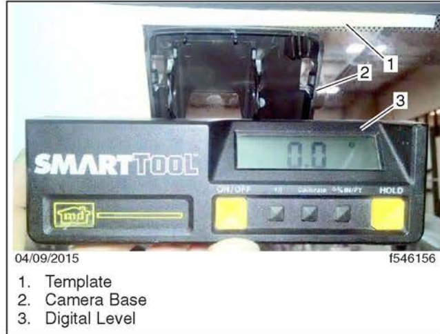
Fig. 11, Aligning the Base with a Digital Level
