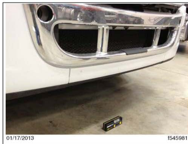
Fig. 6, Measuring the Level on the Surface where the Vehicle is Parked
