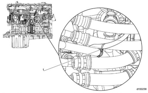
46. Install the chassis fuel feed and return lines on to the fuel filter module. Refer to OEM procedures.
