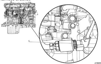
44. Using a zip tie (1), attach the fuel temperature and the LPPO wiring harnesses to the low pressure flange.
