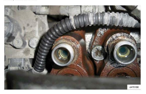
14. Clean the sealing area inside the high pressure fuel rail using a clean, lint-free cloth.
