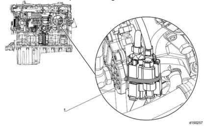
45. Using a zip tie (1), attach the LPPO wiring harness H-clip to the coolant line.
