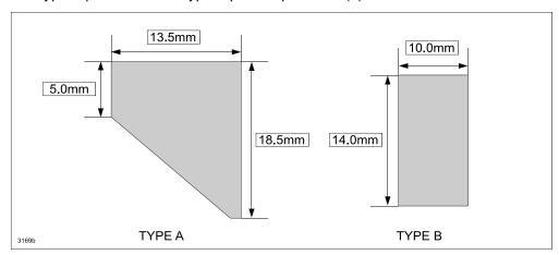
3. First, apply the Type A piece to the upper rear corner of the new run channel (as shown below), then apply the Type B piece.
