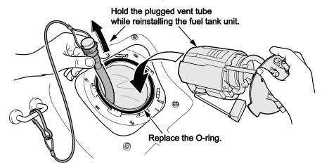
3. Remove the plug away from the tank opening and connect the tube to the fuel tank unit.
