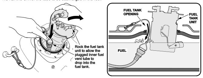
6. Remove the fuel tank unit.
