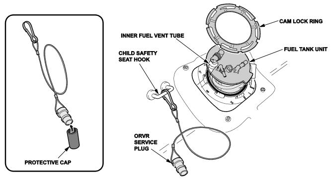
3. Disconnect the inner fuel vent tube from the fuel tank unit and hold it. Do not allow the tube to drop into the fuel tank.
