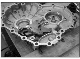
71. To make component installation easier, level the side cover with wood block(s).
