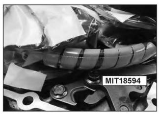
48. To prevent damaging the belt during further steps, wind 28" protective tubing (MIT18594) around its entire length.
