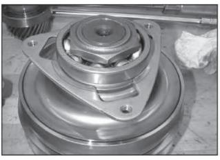
63. Thread the new 50mm lock nut (2771A004) in place.
