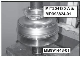
62. Set a new primary pulley bearing (2950A047) in place.
