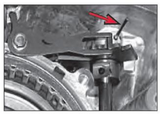
85. Install the manual shaft locating pin.
