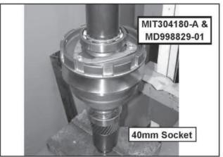
68. Support the output gear on the press table using special tools MIT304180-A and MD998829-01.
