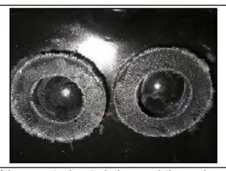
If the magnets show typical accumulation as shown above, reinstall the pan and perform this TSB to replace the pulley bearings.
