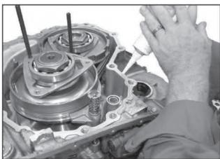
88. Apply a 1.5mm (0.060") bead of Loctite 509 (or equivalent) to the mating surface of the side cover.
