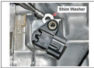
143. Using a stick magnet, hold the shim into position under the secondary pulley speed sensor mounting tab while installing the speed sensor into the transaxle case.
