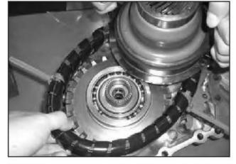
78. Once the belt is in position, install the secondary pulley assembly into the side cover.
