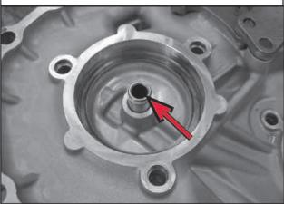
70. Install a new sealing ring (2931A005) as shown here.
