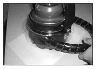
75. Install the belt around the secondary pulley. Note the directional arrow.
