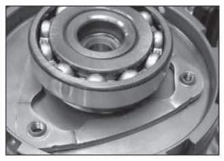
67. Position the new bearing retainer (2771A002) and new bearing (2950A048) onto the secondary shaft as shown here.
