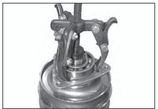
60. Use a common 3-jaw puller (e.g. OTC-1023) to remove the primary pulley's rear bearing. Discard the bearing and bearing retainer.
