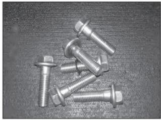
92. Install new o-rings (2791A012) on the six bearing retainer bolts.
