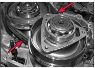
44. Keep the drive belt from separating during further disassembly by securely attaching two tie-wraps around the belt at the locations shown by the arrows.
