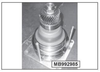
65. Position the secondary pulley assembly (lock nut down) in the holding fixture (MB992985) as shown
