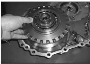
72. Install the primary pulley into the side cover.
