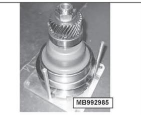
69. Thread a new 50mm lock nut (2771A003) onto the shaft and return the secondary pulley assembly to the holding fixture (MB992985) as shown.
