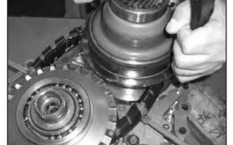
Like the primary pulley installation, shake the assembly until the bearing is seated.
