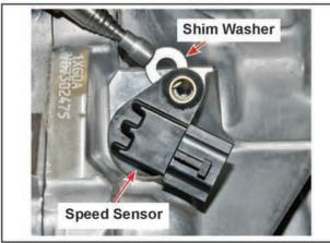
At the same time the secondary pulley speed sensor is being removed from the transaxle case, using a stick magnet to remove the secondary pulley speed sensor shim washer.
