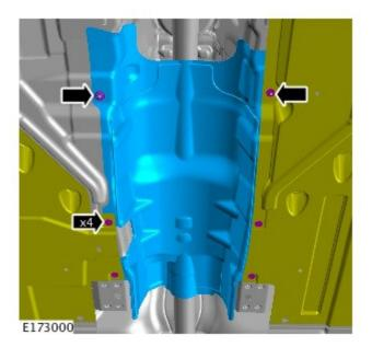
**3.** Remove the cross brace and fixings.
