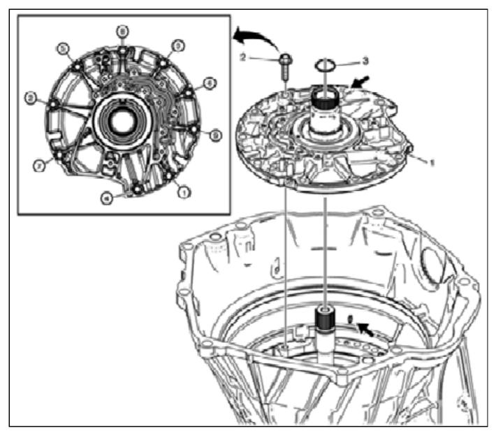
**Note:** Align the bolt hole indicated by the arrow with the arrow that is cast into the case and push down to seat.
