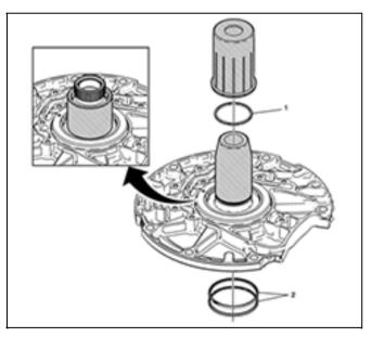
(B) New stator support asm
