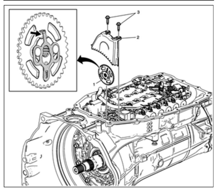
**Note:** Ensure the driven sprocket locking tab is in the unlocked position before installing the sprocket. The driven sprocket locking tab is located on the back of the sprocket and faces the pump.
