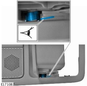
12. ONOTE: Use care when installing the sunglasses holder cover or the sunglasses bin will not function correctly.
