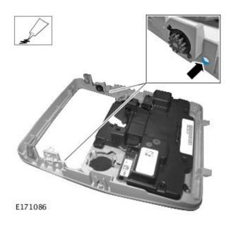
6. Rotate the cam latch through 360 degrees whilst visually inspecting it for possible damage.
