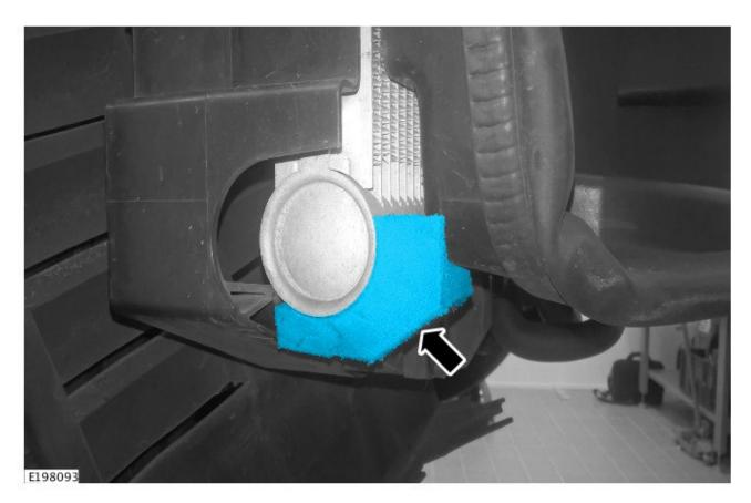
**6.** Install the new foam pad to the inner edge of the auxiliary radiator as shown.
