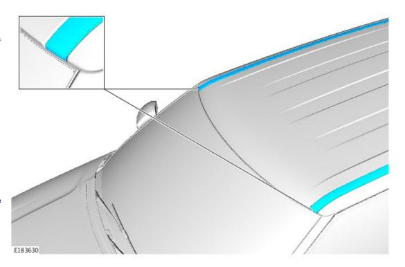
hold down the roof moulding in the area shown.
