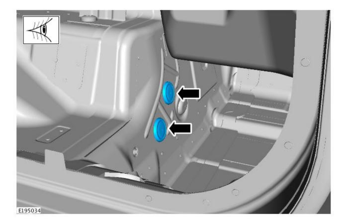
**5.** Install the grommets as shown.
