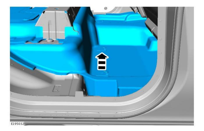
4. Visually check to see if the grommets are installed.
