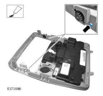
6. NOTE: Make sure the spring is positioned correctly.
