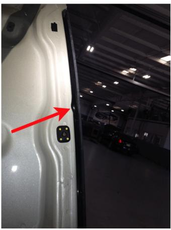
2. Install a 5mm X 5mm (3/16 X 3/16) piece of closed cell foam tape along the entire length of the tail light assembly, as shown below.
