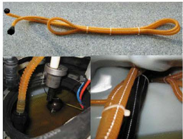
Figure 1. The long, curved fuel lines that run across the fuel tank from right to left.
