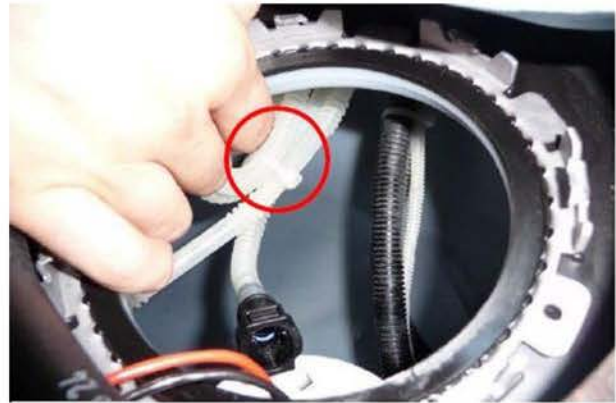
Figure 6. Curved fuel lines, fuels supply pipe, and fuel line tied together with tie wrap.
