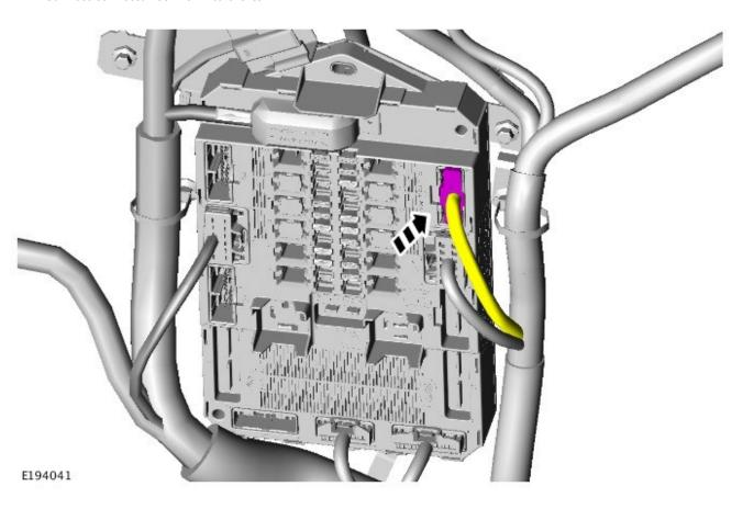
15. NOTE: If the vehicle does not have a towbar fitted, this connector is not used. If the vehicle has a towbar fitted, this connector must be disconnected and the new harness connectors installed inline.
