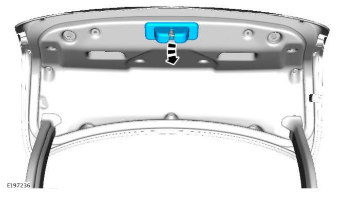
**10.** Install the two fasteners.
