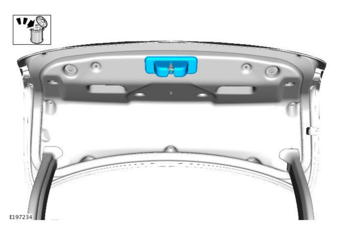
**5.** Pull the luggage compartment lid carpet trim down as shown and visually check that the latch assembly clipping features are intact and not damaged.
