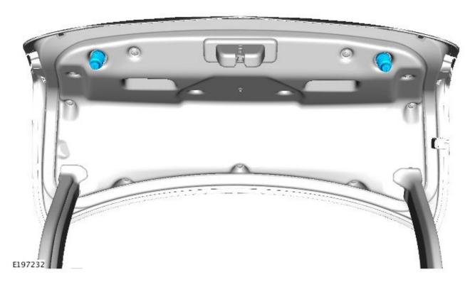
**3.** Remove the two fasteners.
