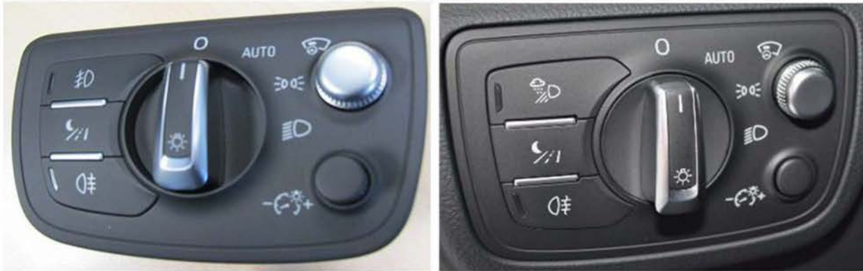
Figure 3. A6 and A7 headlight switch knob pushed in (left) and in normal position (right).
