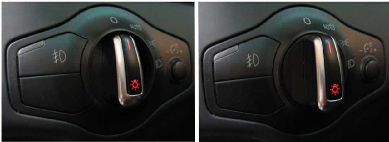
Figure 1. B8 headlight switch knob pushed in (left) and in normal position (right).
