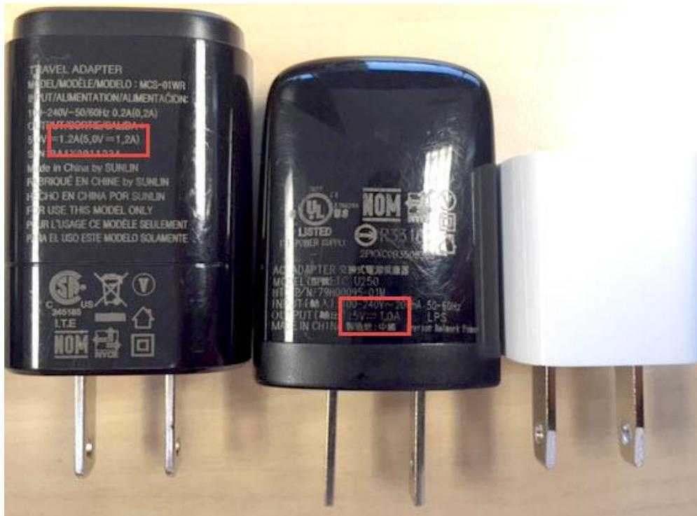
*Figure 3. USB Smartphone charger with 1A current supply capability.*
