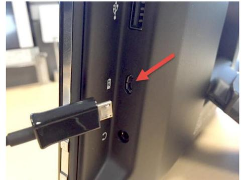
*Figure 2. Micro USB charge port.*
