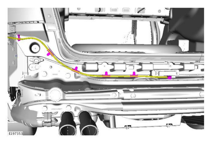
**9.** Remove the rear bumper support bracket.
