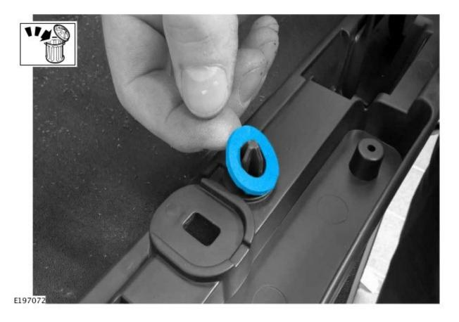
**12.** Using a suitable tool, remove the section of the Y center locator flush with the base as shown in blue. The remaining piece of the Y center locator should be 5mm as shown.
