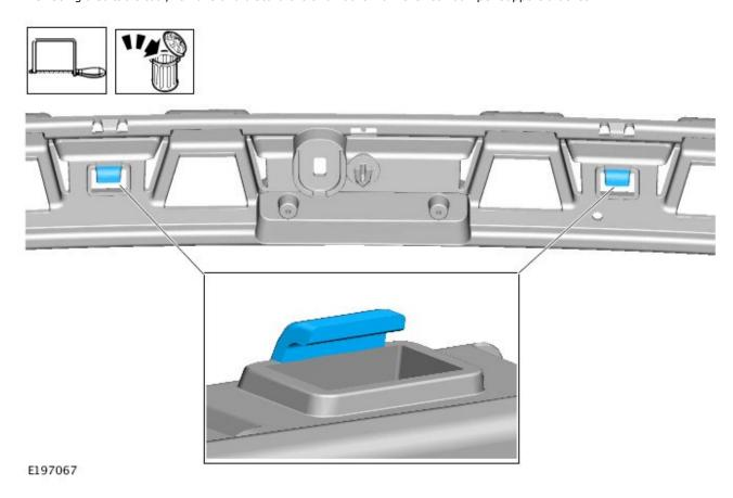
**11.** Remove and discard the foam washer from the Y center locator.
