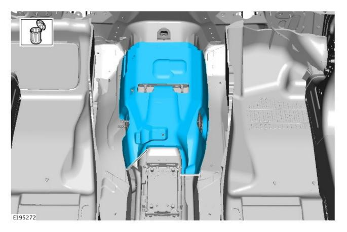
**8.** Using the removed tunnel insulation cover that was removed in step 7 as a template, cut the replacement tunnel insulation cover as shown.
