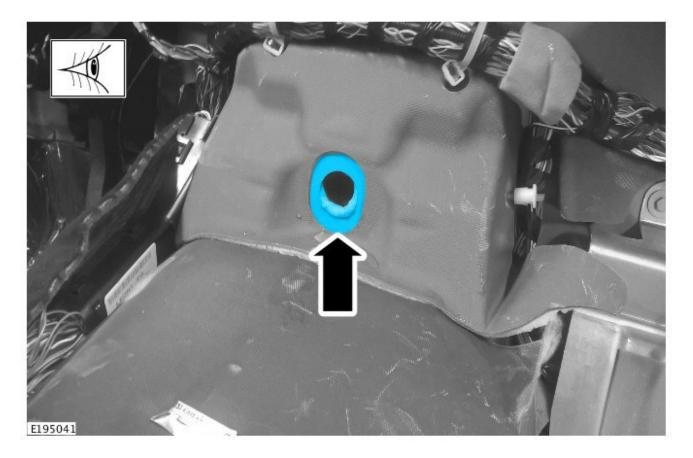
4. **ONOTE:** Once the seal has been broken, do not insert the suitable tool any further. Inserting the suitable tool any further into the drain tube may damage the transmission heatshield.
