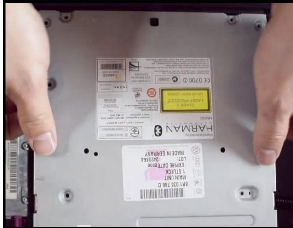
Figure 7. Pry top cover off with fingers.
