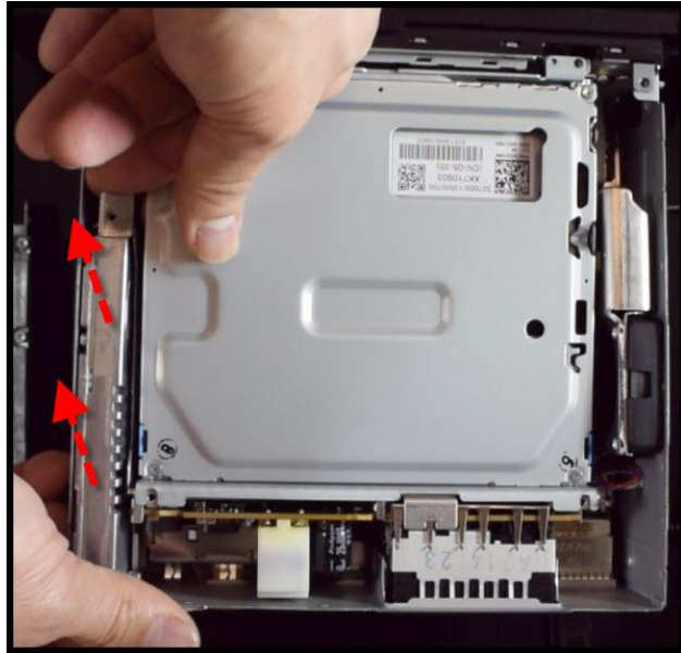
Figure 11. Lift up on both ends of the telephone module as indicated by the red arrows.
