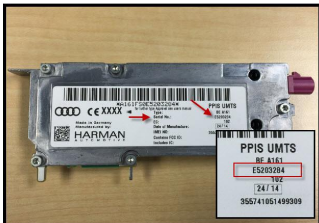
Figure 12. Serial number of the PPIS UMTS telephone module indicated by the red arrows and red box.
