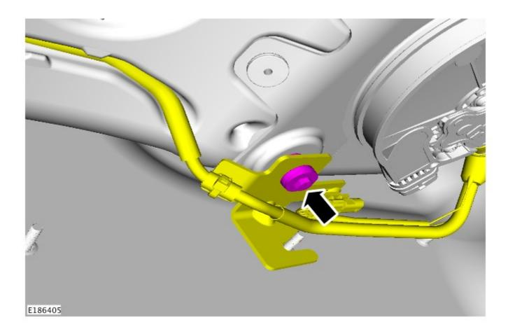
10. Install the diesel exhaust fluid tank support bracket securing nut.
