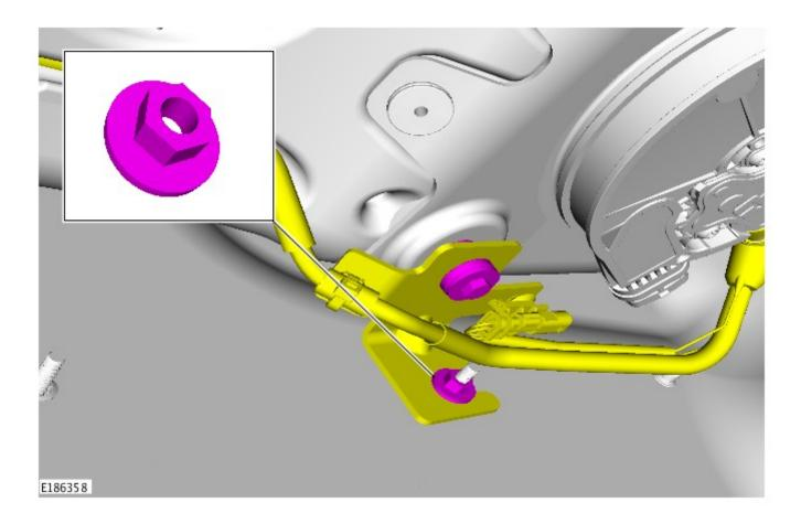
4. NOTE: When the bolt has been removed, the support bracket will move aside.
