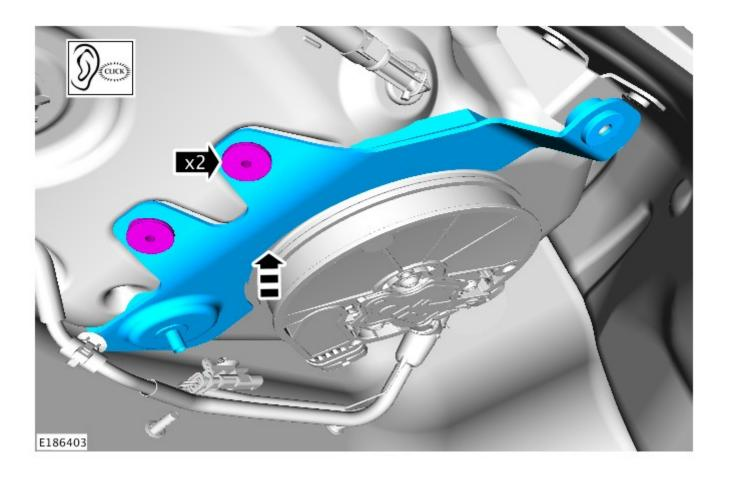
8. Install the modified diesel exhaust fluid tank lower bracket bolt.
