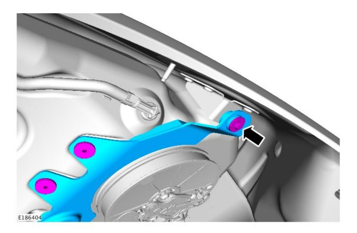
**9.** Install the diesel exhaust fluid tank support bracket securing bolt.
