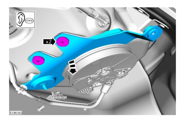
${\bf 7.}$  Install the modified diesel exhaust fluid tank lower bracket.
