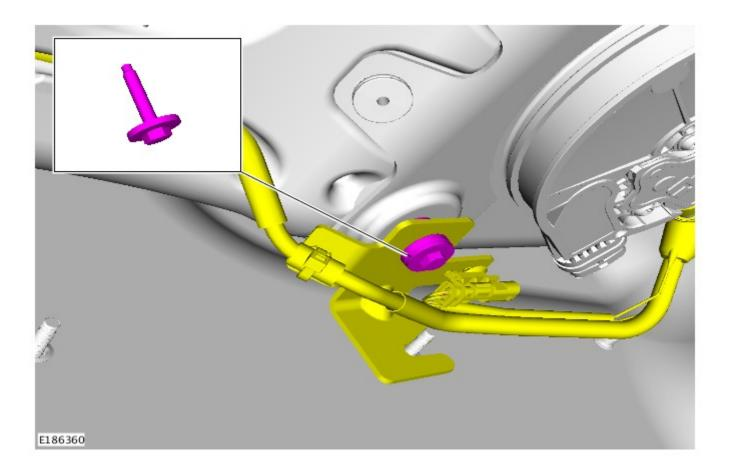
**5.** Remove the bolt holding the diesel exhaust fluid tank lower bracket in place.
