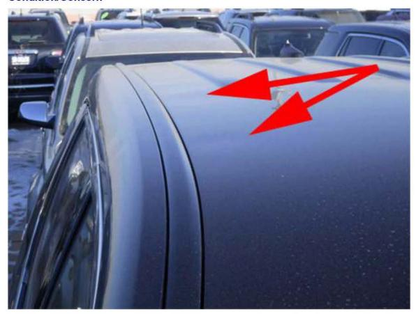
Some customers may comment on denting or waviness along the outer edges of the roof panel near the roof panel moldings (ditch moldings). This is caused by the welding process of the roof panel to the side door (closure) panel.
