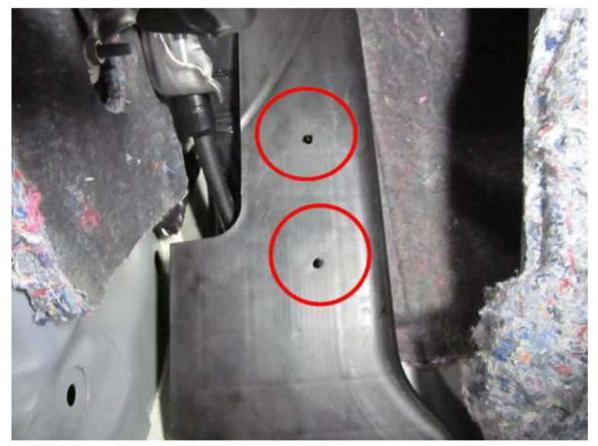
6. Install the footrest and the two mounting nuts.
