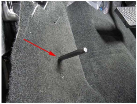
9. Lift the carpet back up, remove the rivets and use a punch to open the holes of the carpet to allow push pins through.
