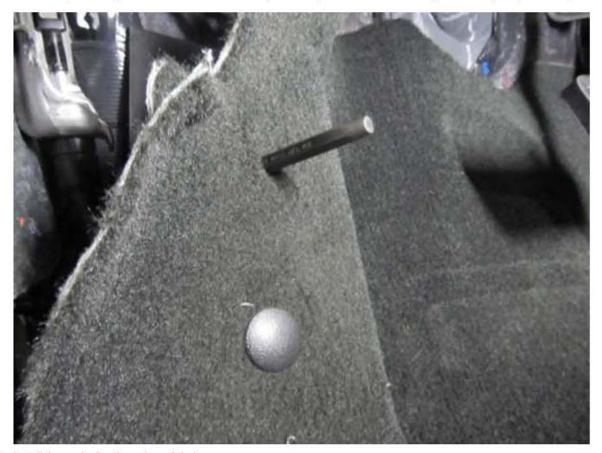
Install the push pins through each hole.
