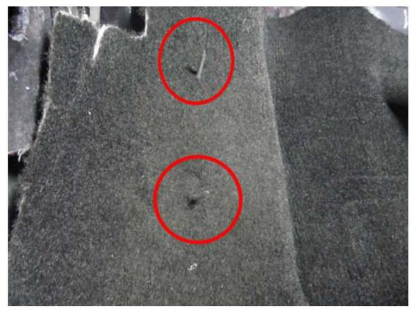
8. Push the carpet over the rivets and punch through the carpet as shown.
