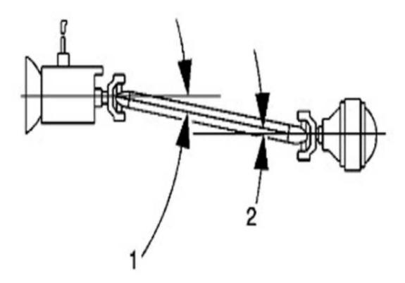
Propeller systems containing only 1 U-joint: The U-joint working angle should be between 1/2 and 3/4 degrees.
