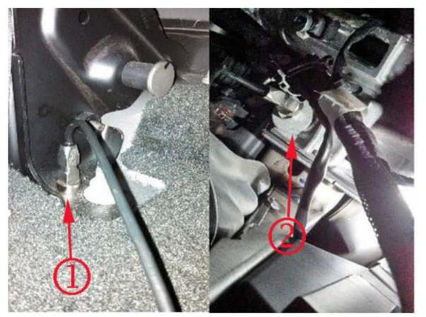
3. Using a Pico Oscilloscope Diagnostic Kit, mount the PicoScope vibration sensor on one of the two locations shown above.
