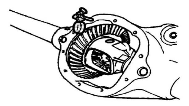
2. Install the J-25025 pins and the J-8001 indicator to the axle housing.
