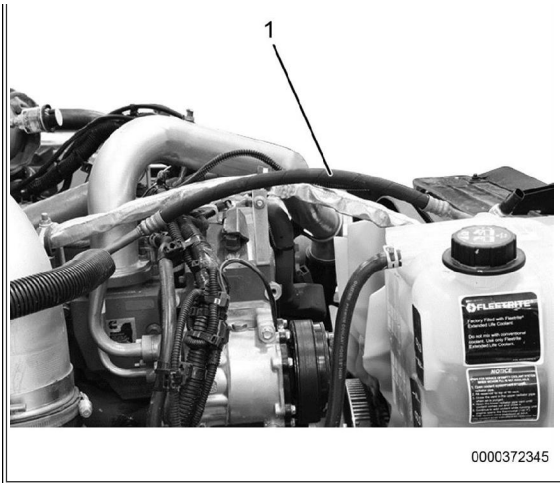
Figure 7: A/C Compressor Discharge Line - Cummins Equipped ProStar 122.
