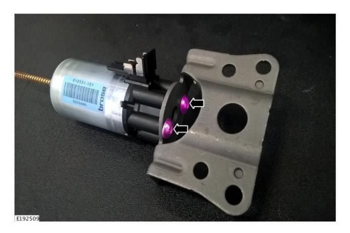
3. NOTE: The orientation of the front seat track motor to the bracket must be installed as shown ( / ).
