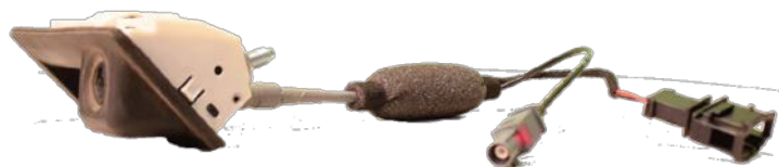
Figure 2. Reverse camera harness to be replaced.
