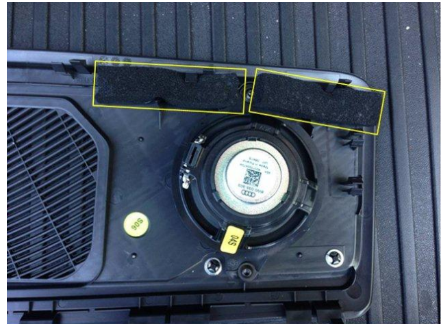
Figure 2. Foam strip installation for vehicles with Bang and Olufsen (PR code 9VS).
