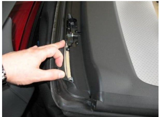
Figure 4. Lifting the corner.
