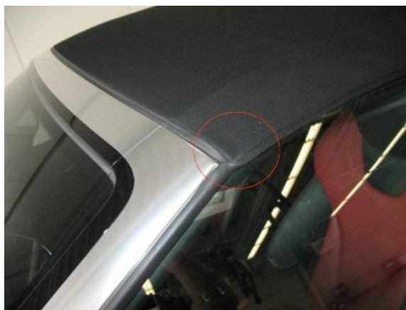
Figure 1. Location where a leak may occur.
