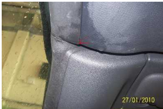
Figure 2. Evidence of a leak.
