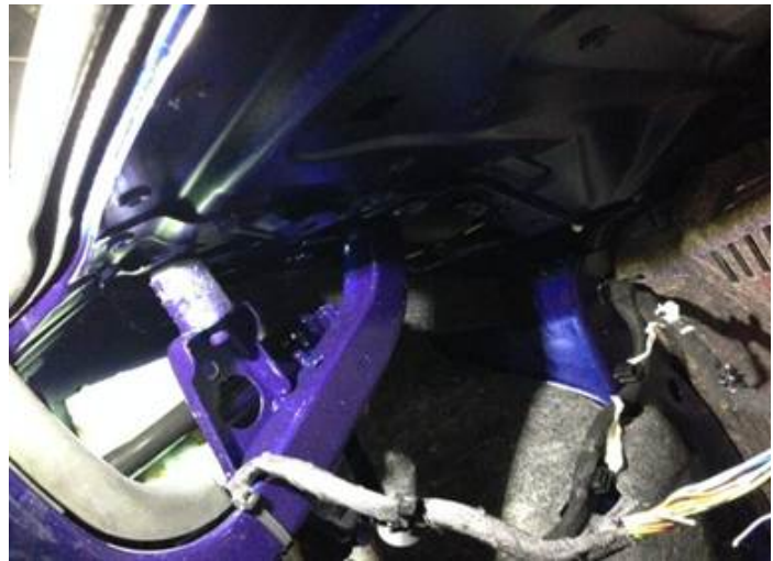
Figure 3. Incorrect wire routing at trunk hinge.
