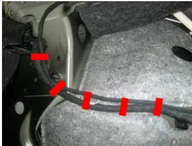
Figure 8. Wrap the wiring harness with textile adhesive tapes at red marks.
