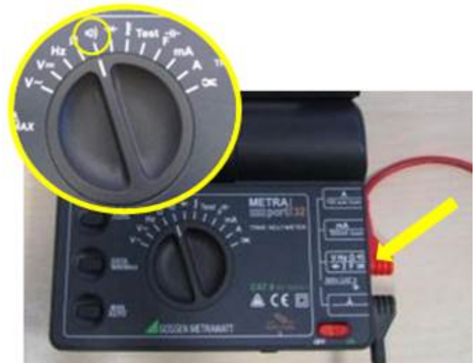
Figure 12. Set the VAG 1526 C to current flow check and connect the probe cables.
