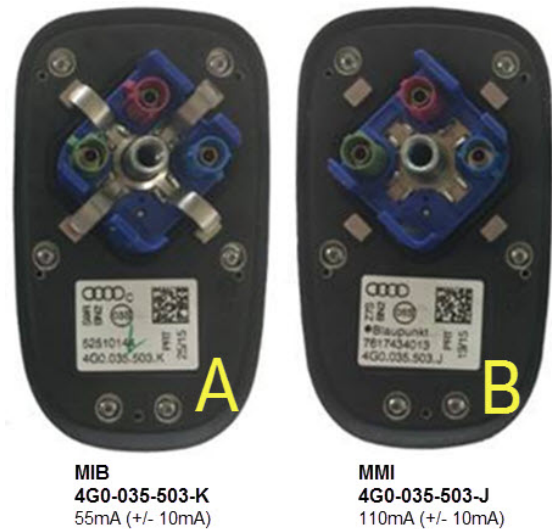
Figure 2. MIB antenna with K suffix part number 4G0-035-503-K (A), and MMI antenna with J suffix part number 4G0-035-503-J.
