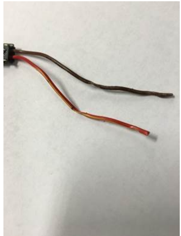
Figure 5. Damage typically found on roof harness.
