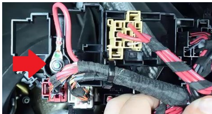
Figure 26. 10mm nut to be removed from the bottom of fuse panel B -SB-.
