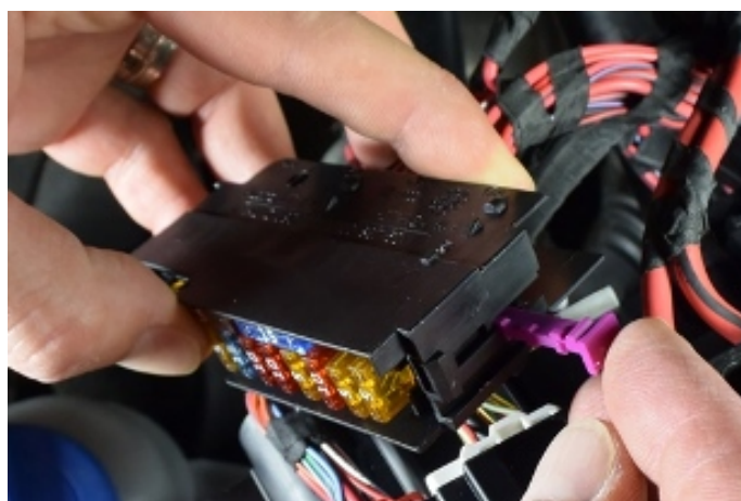
Figure 24. Reinstalling the terminal lock in to the fuse block.
