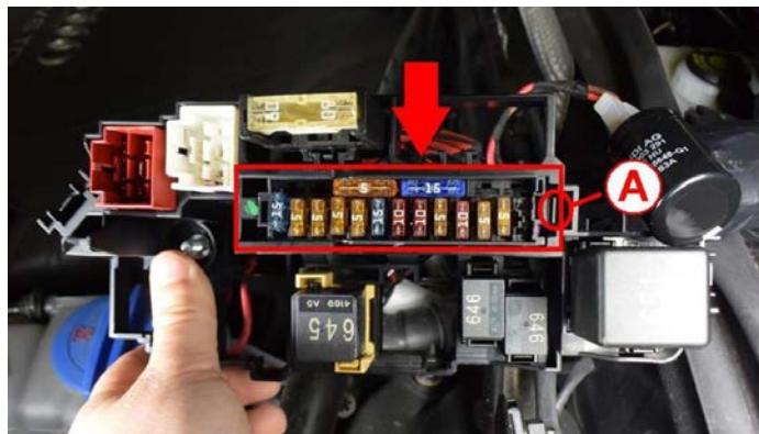
Figure 9. Fuse block ST1 with tab for removal (A).
