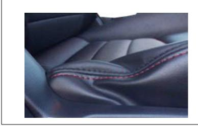
Example of collapsed front passenger side support
