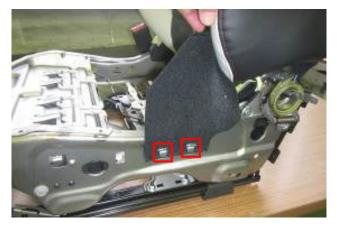
b. Install the hook (A) of the mat on the spring (B) from the bottom side.
