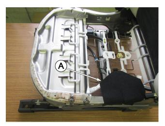
a. Attach the holes of the mat to the hooks on the side frame.
