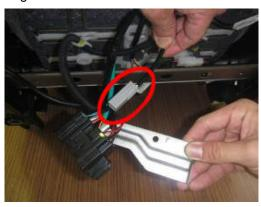
**NOTE:** Take care not to damage the connector clips (A) when removing the connector from the hole.
