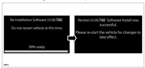
30. After the update is completed with the above right screen, confirm that the push button start indicator light is illuminated (amber) and the display in the instrument cluster is OFF (ignition is in "ACC"). If the ignition is "OFF" and the push button start indicator light is not illuminated (amber), turn the ignition to "ACC" and one of the following two screens will be displayed.
