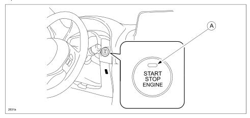
**NOTE:** The engine starts by pressing the push button start while depressing the clutch pedal (manual transaxle) or the brake pedal (automatic transaxle). To switch the ignition position without starting the engine, press the START/STOP ENGINE push button without depressing the pedal.
