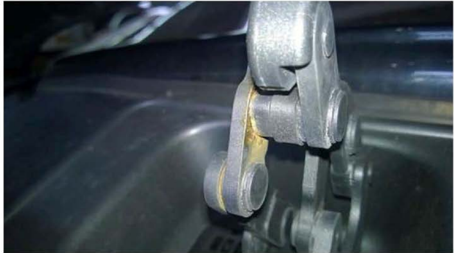
Figure 1. Corrosion on the spoiler drive unit hinge.
