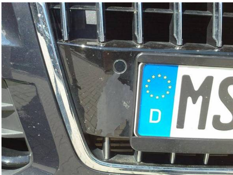
Figure 1. Example of flaked-off paint.
