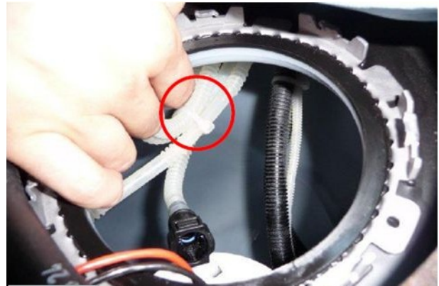
Figure 6. Curved fuel lines, fuels supply pipe, and fuel line tied together with tie wrap.
