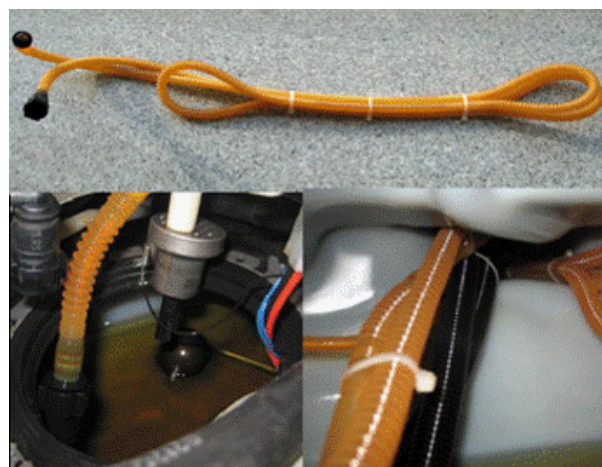
Figure 1. The long, curved fuel lines that run across the fuel tank from right to left.
