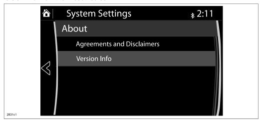
4. Make sure the software version is 56.00.760 or later, then select OK. If it is not 56.00.760 or later, update the system using a USB memory stick with the latest software according to the "Reflash Procedure." If needed, refer to "Downloading Update Software to a USB Memory Stick (for additional USB memory sticks)" below.
