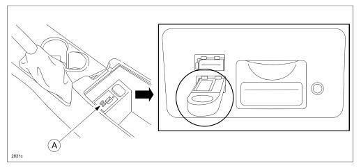
**NOTE:** There should only be the prepared USB memory stick inserted in one of the USB ports. Nothing else should be inserted in the other USB port during the re-flashing process.
