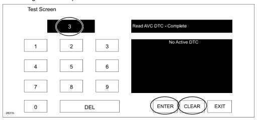
10. Whether any DTCs are present or not, input '2' on the test screen and then select "ENTER". This will internally clear all the earlier set DTCs (in the CMU). Select "CLEAR" to go to next step.
