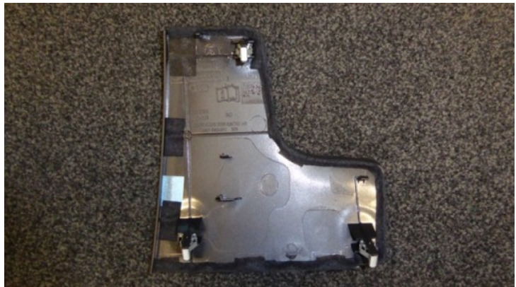
Figure 5. Fuse panel 'C' cover.
