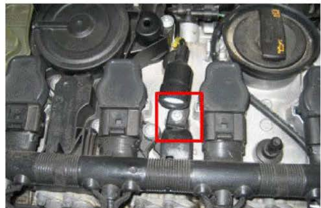
Figure 3. Securing bolt for engine wiring in in-line engine.
