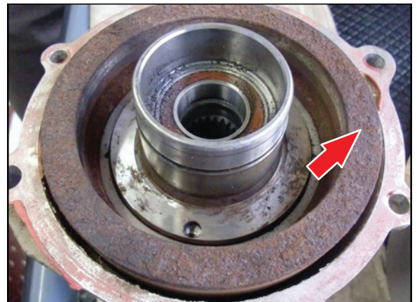
Figure 9. Excessive Rust/Corrosion Buildup on Edge of Coupling Body
