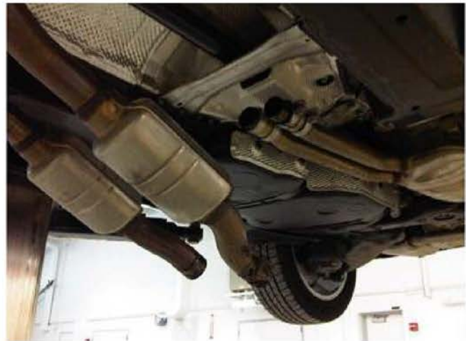
Figure 4. Lowered catalytic converter pipes
