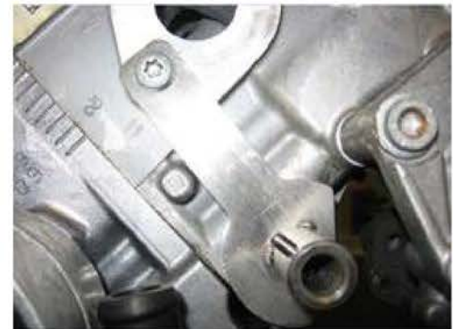
Figure 11. Engine adaptor on bank two.
