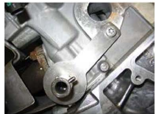
Figure 10. Engine adaptor on bank one.
